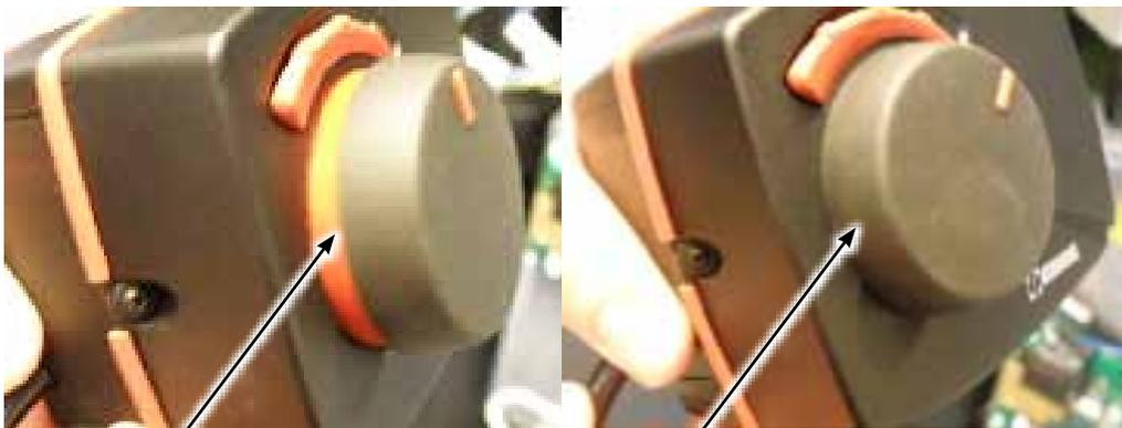
Manual mode when the button is not pressed in. Auto when the button is pressed.
