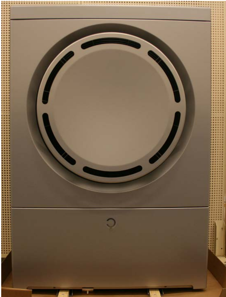
Figure 1 Heat pump, outdoor unit
